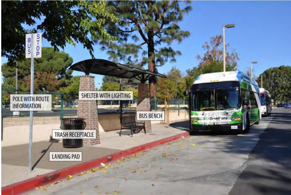
**Figure 3-4: Standard Omnitrans Local Bus Stop**
