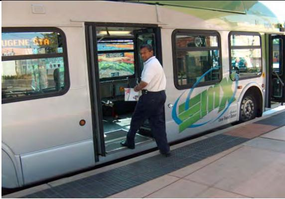
Level Boarding – Similar to rail systems, low floor vehicles and taller station platforms that provide level boarding speeds up the boarding and disembarking processes, especially for wheelchair-bound passengers.
