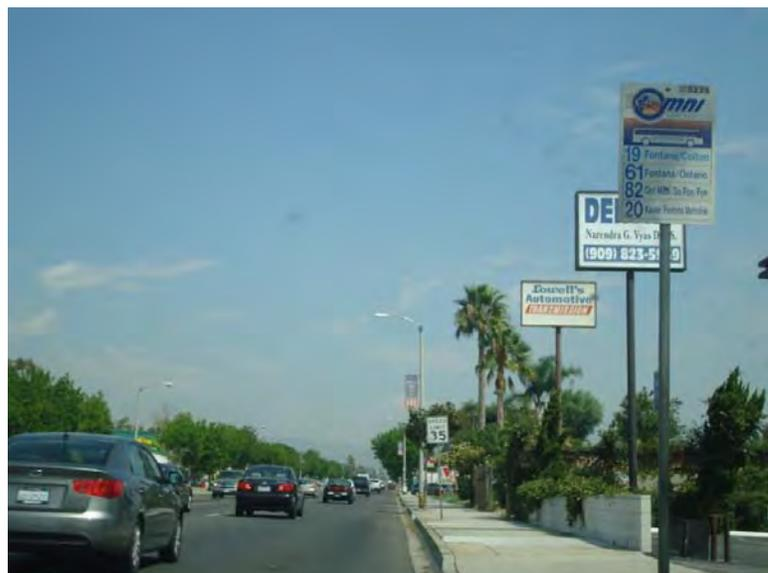
Avenue, Foothill Boulevard consists of two lanes in each direction with a two-way painted median and on-street parking provided via a wide curb lane. The posted speed limit is 55 miles per hour in both directions on the western portion of the route, transitions to 50 miles per hour, then to 45 miles per hour on the eastern portion between Almeria Avenue and Sierra Avenue.
